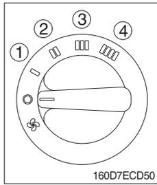
(1) It is possible to control the fan speed to four steps.
