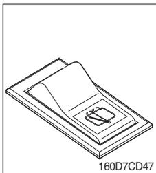
(1) This switch is used to operate the rear wiper and washer by two steps.
