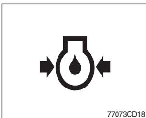
① This lamp comes ON for a while after starting the engine because of the low oil pressure.
