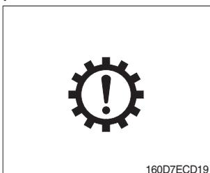
① This lamp lights ON and the T/M message display shows the error codes when an error occurs in the transmission.
