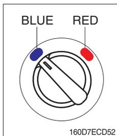
(1) This switch regulates the temperature of air.
