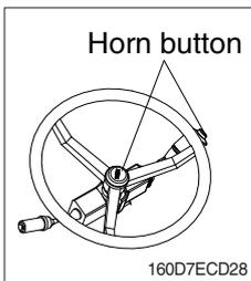
(1) If you press the button on the top of the multifunction switch and the center of the steering wheel, the horn will sound.
