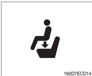
① This signal lamp lights ON when the operator leaves the seat.
