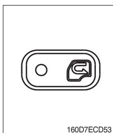
(1) If this switch is pressed, air from the outside is inhaled
