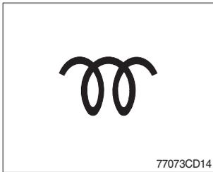
① This lamp lights ON when start switch is turned clockwise to the ON position. Light will turn off after approximately 15~45 seconds, depending on engine coolant temperature, indicating that preheating is completed.
