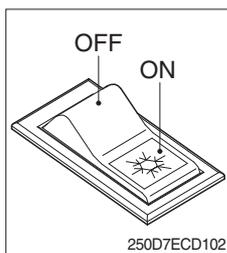
(1) This switch is used to turns ON or OFF the air conditioner.
